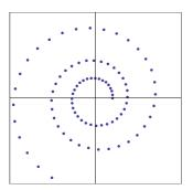
Nonholonomic integrators are sensitive to how the constraints are discretized. For instance a trajectory of the contact point of a discrete balanced Chaplygin sleigh (a platform supported by a skate) may become a spiral, which is not what the continuous-time model predicts
