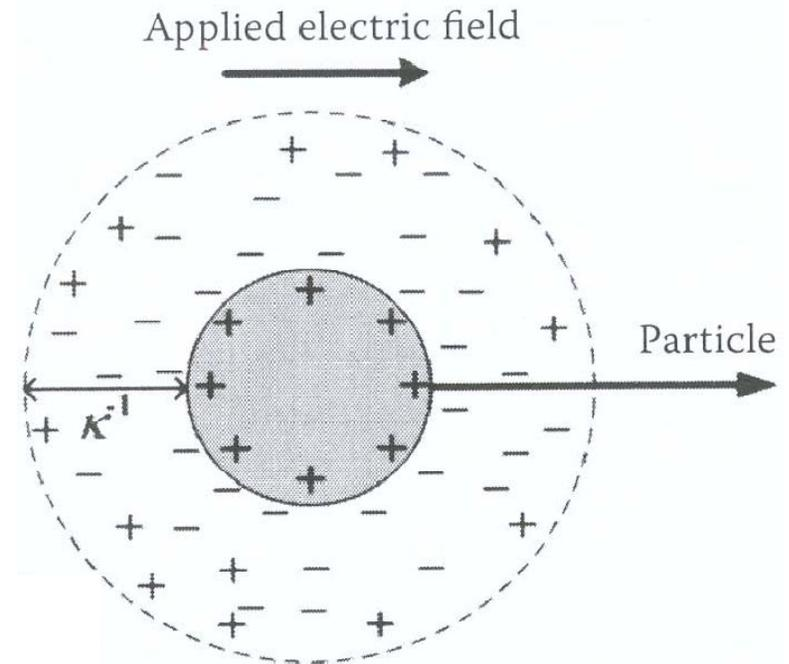
Electrophoresis : Motion of charged particles in solution due to electrical field.
