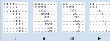
Figure 7: Steps of Binary Skeletonization
