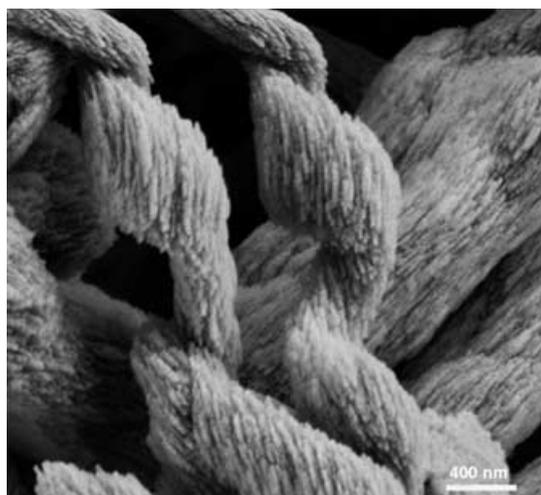
**Figure 20.** SEM image of helical BaCO<sub>3</sub> fibers formed in presence of a stiff phosphonated block copolymer. Reproduced from ref. [84] with permission of Nature Publishing Group.
