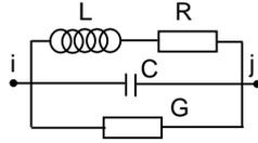
**Fig. 2** High frequency branch between two nodes
